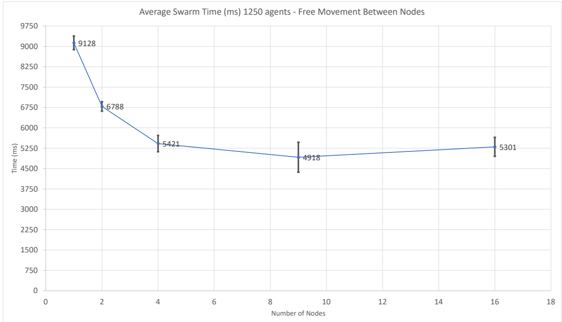
Figure 6.4: Swarm timing (ms) for 1,250 agents on 1, 2, 4, 9, and 16 nodes, using data from Chapter 4 with cellular morphology features, with agents moving freely between nodes, averaged over 25 runs. Error bars represent standard deviation.
